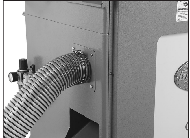
Figure 13. Dust hose attached to dust port.
